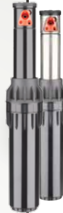
I-35-06: Overall height: 10 \frac{3}{8} " Pop-up height: 6" Exposed diameter: 1 \frac{1}{8} " Inlet size: 1" female NPT
