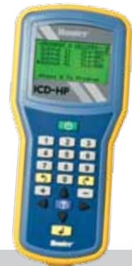
ICD-HP: Handheld programmer
