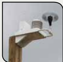
Local ET Sensor, includes Rain Gauge
