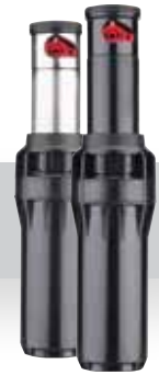
I-25-04: Overall height: 7 7/8" Pop-up height: 4" Exposed diameter: 1 1/4" Inlet size: 1" female NPT
